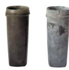
No corrosion with Rapid corrosion of Alocrom treatment. untreated aluminium.
